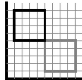
$$\begin{aligned}x' &= x + t_x \\y' &= y + t_y\end{aligned}$$
